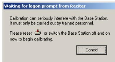
5. When the TB9100 Calibration Software program has successfully connected to the reciter (this can take up to 30 seconds), the Calibration Wizards are displayed in the main window.
